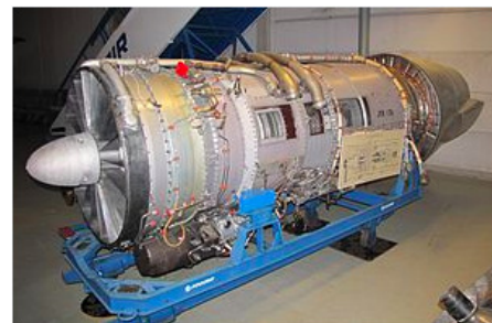
Figure 1. The JT8D is a low-bypass turbofan often used on early narrowbody jetliners.
